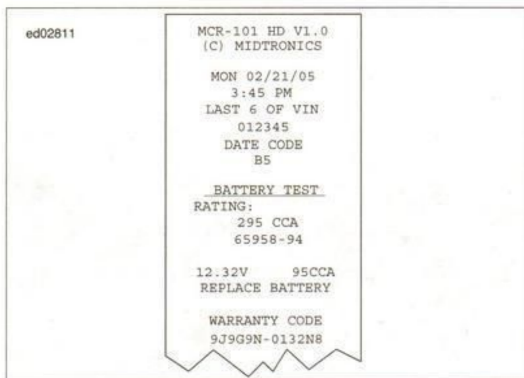
Figure 3-19. Battery Test Results Printout
