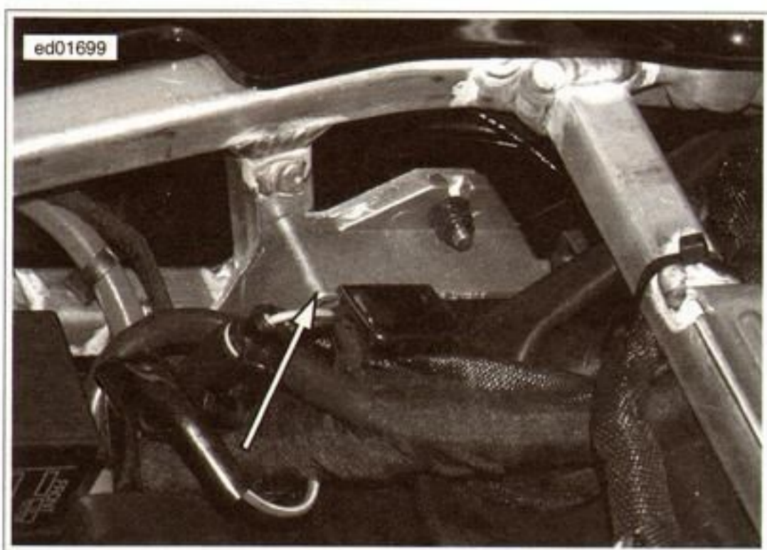
Figure 3-11. Voltage Regulator Location
