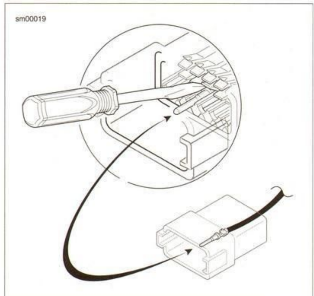
Figure A-14. Deutsch Connector: Depress Terminal Latch and Back Out Pin
