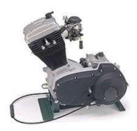
The 492cc engine uses a Sportster-derived, but much lighter, lower end and connecting rod attached to a standard 1203cc Buell piston. The cast, high-pressure permanent mould engine cases are specific to this motorcycle. The casting method used on these cases allows for a varying wall thickness (as opposed to die casting). This was necessary to provide sufficient strength in specific areas such as where the swingarm attaches. A plus with these cases is the accessibility of the oil filter.
