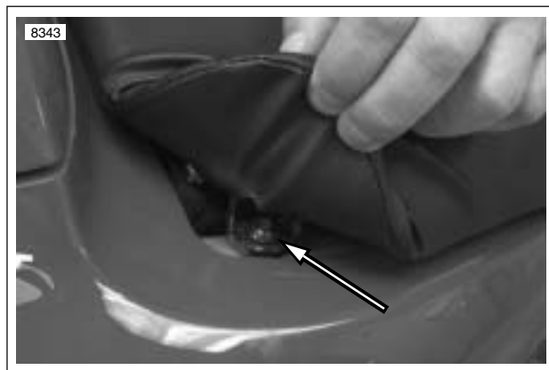
Figure 2-120. Accessing Rider Seat Screws
