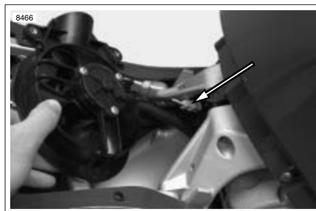
Figure 4-83. Cooling Fan Connector [97]
