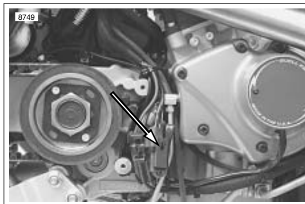
Figure 4-64. Cam Position Sensor Connector [14] (stator connector disconnected)
