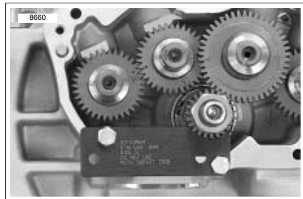
Figure 3-128. Crankshaft Locking Tool (Part No. HD-43984)
