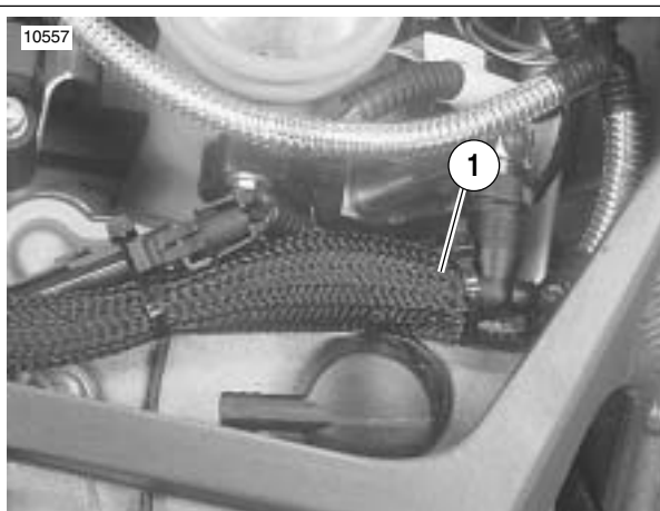
1. Engine temperature sensor connector [90] (approximate location)
