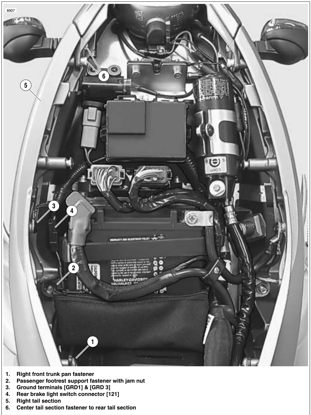
Figure 2-115. Right Side Frame Section
