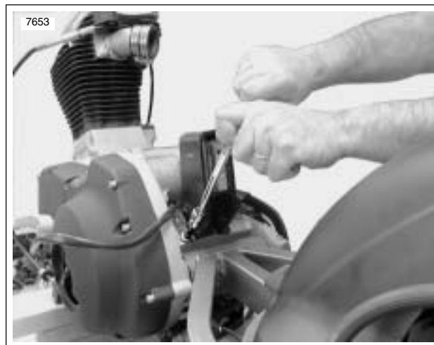
Figure 3-24. Rear Engine Mount
