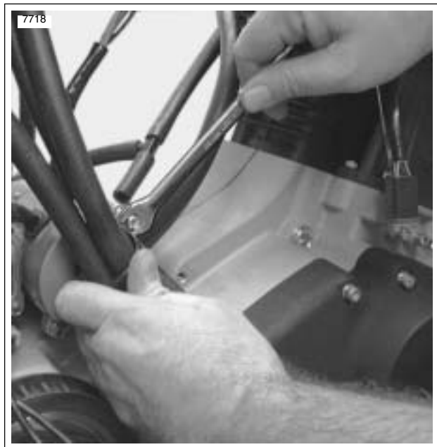
Figure 3-31. Tighten Clamp
