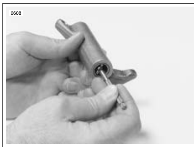
Figure 3-54. Measuring Rocker Arm Bushing Inner Diameter
