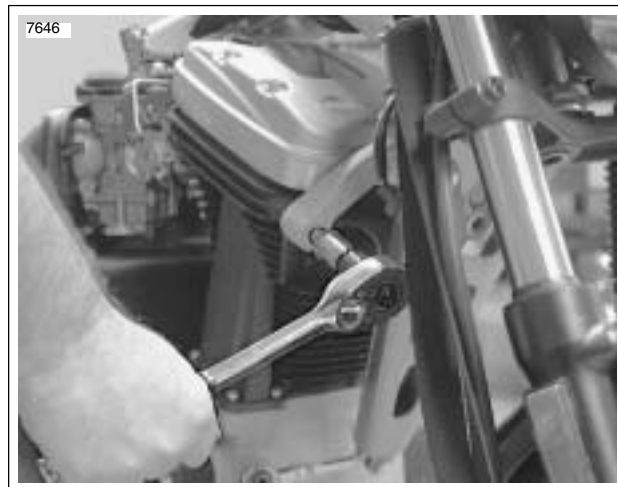
Figure 3-40. Cylinder Head Bolt
