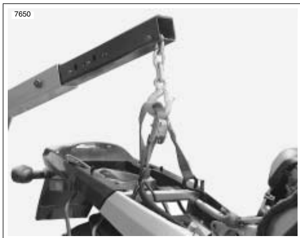
Figure 3-11. Hoisting Bike
