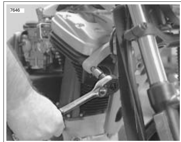
Figure 3-2. Cylinder Head Bolts
