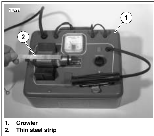
Figure 5-20. Shorted Armature Test Using Growler
