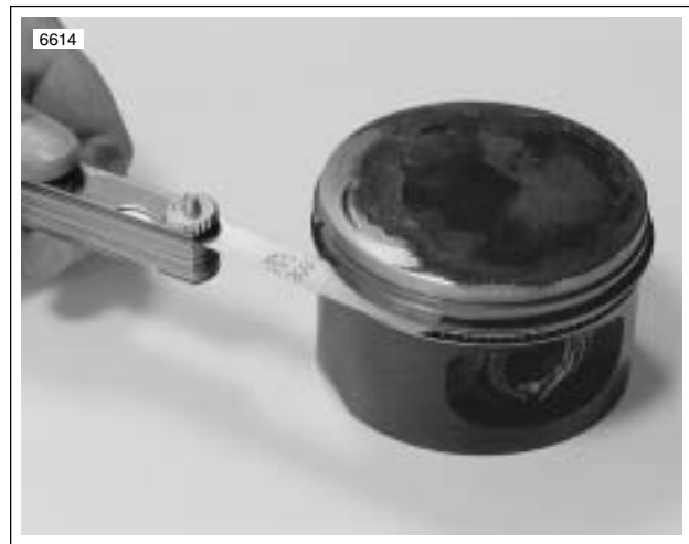
Figure 3-79. Measuring Ring Clearance in Groove
