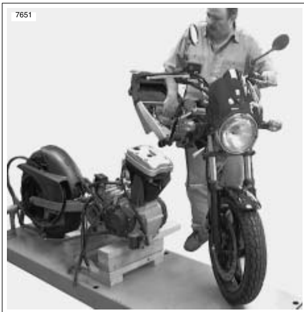
Figure 3-26. Move Chassis to Engine
