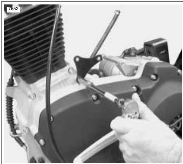
Figure 3-25. Bracket, Left Side Air Cleaner
