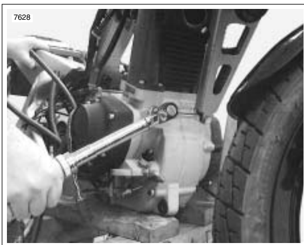
Figure 3-39. Install Front Tie Bar
