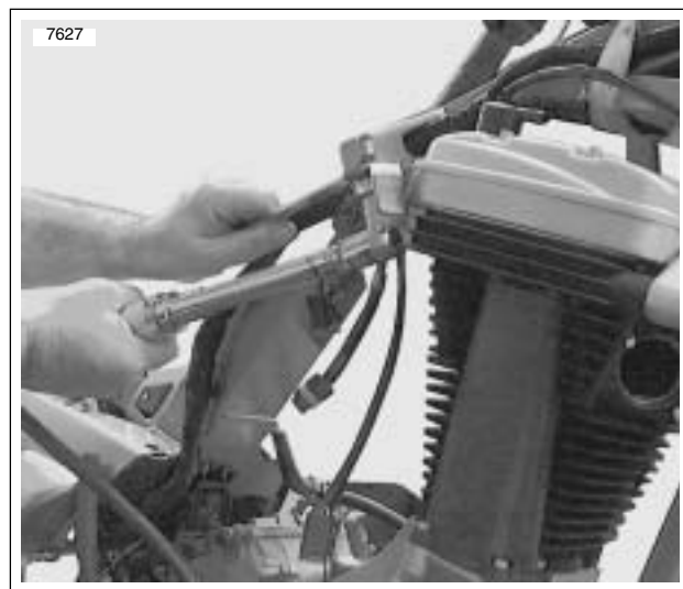
Figure 3-4. Remove Top Rear Tie Bar
