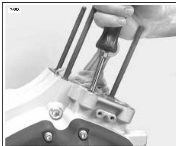
Figure 3-110. Checking Cam Gear End Play
