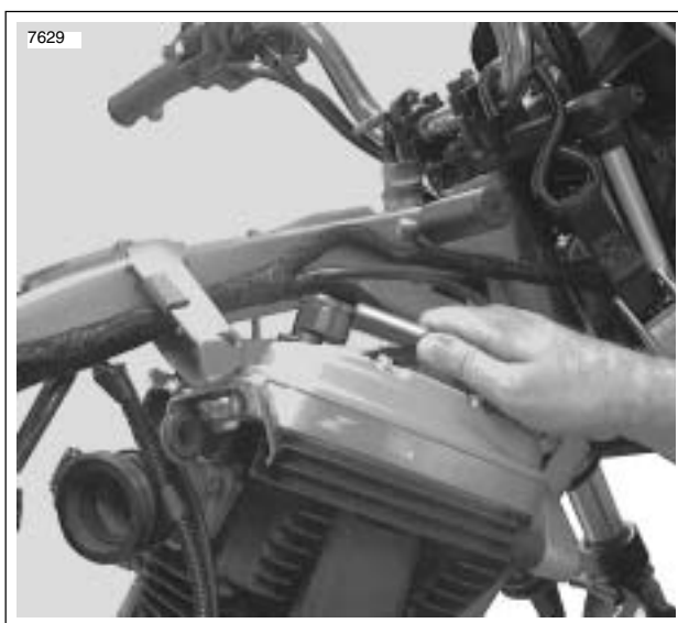
Figure 3-1. Remove Crankcase Breather Hose
