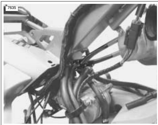
Figure 3-30. Tighten Hose Clamps
