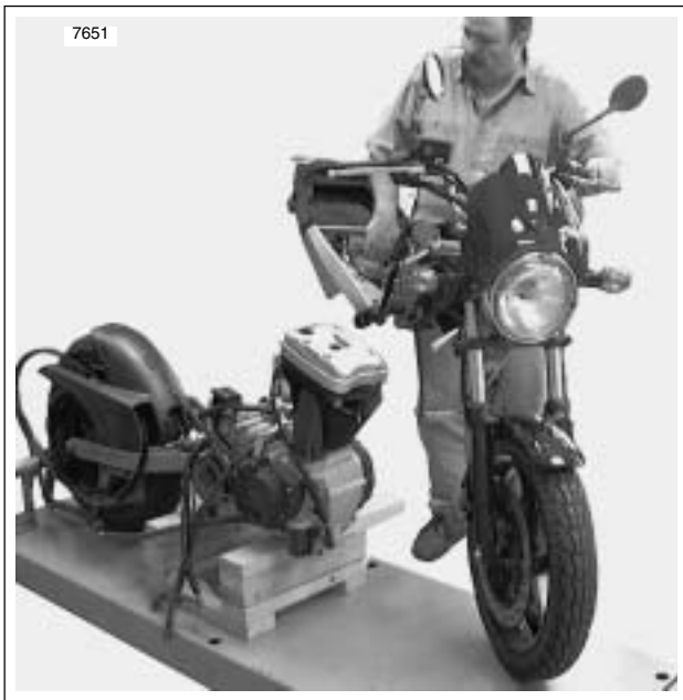
Figure 3-15. Move Chassis From Engine
