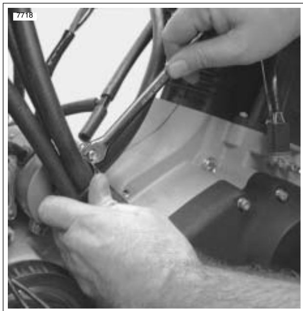
Figure 3-12. Loosen Clamp
