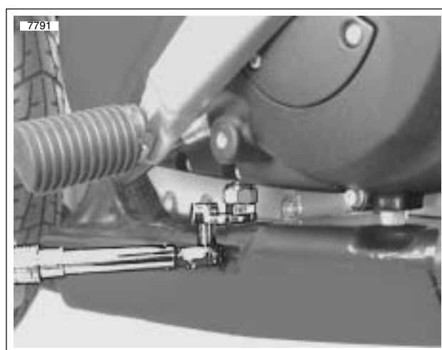
Figure 6-6. Torquing Chain Limiting Screw
