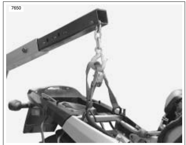
Figure 3-27. Hoisting Bike
