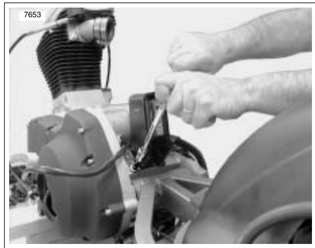
Figure 3-17. Rear Engine Mount
