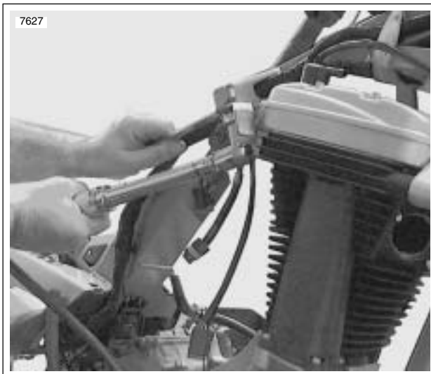
Figure 3-38. Install Top Rear Tie Bar
