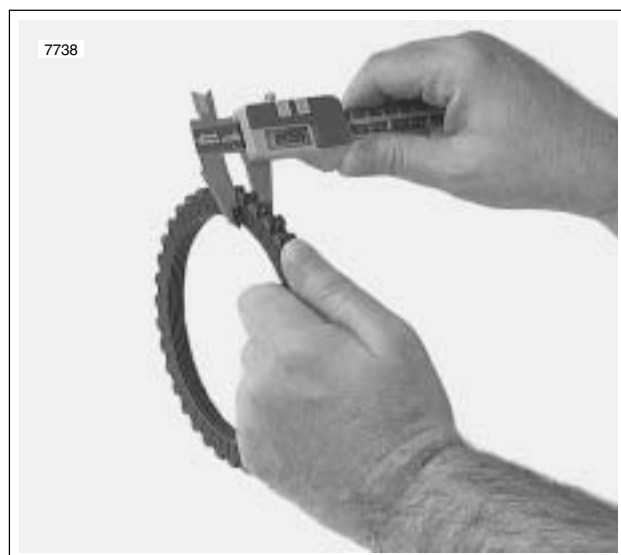
Figure 6-17. Measuring Friction Plates
