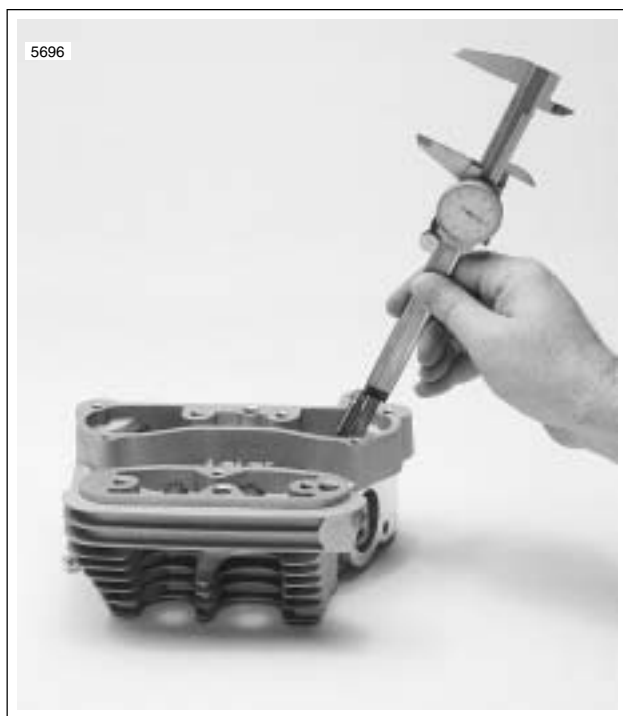
Figure 3-55. Measuring Valve Stem Protrusion
