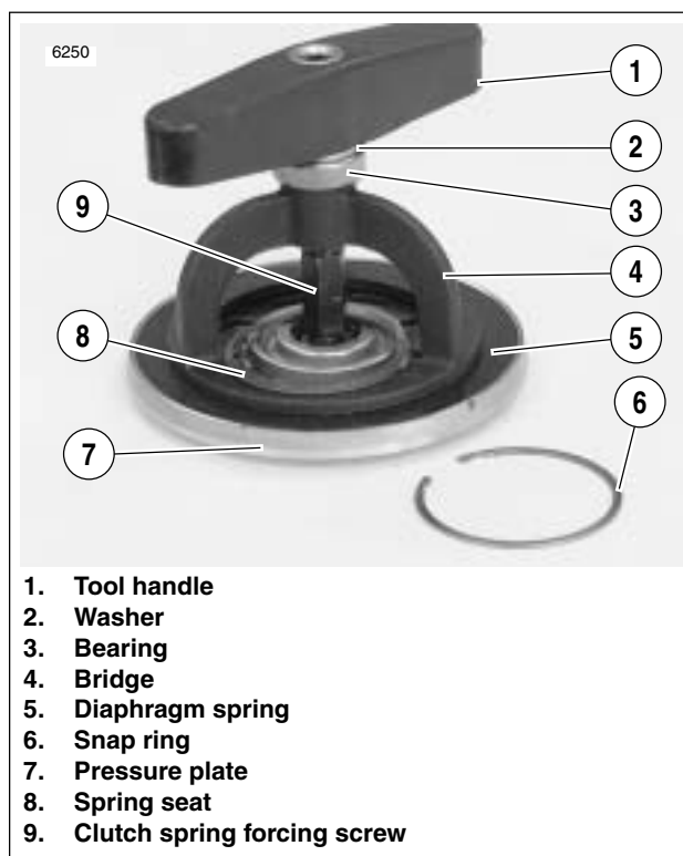
Figure 6-13. Pressure Plate Assembly
