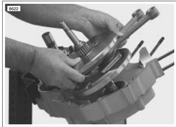
Figure 3-136. Removing Flywheels from Left Crankcase
