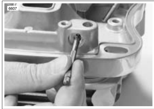
Figure 3-65. Measuring Rocker Arm Shaft Bore Diameter in Lower Rocker Cover (Typical)
