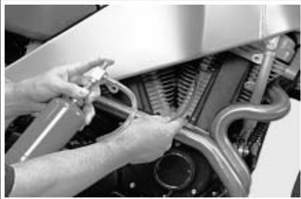
Figure 4-112. Checking for Intake Leak
