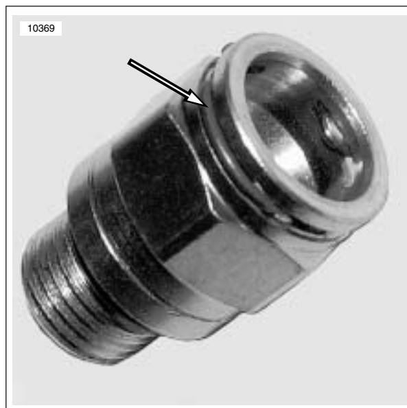
Figure 3-108. Oil Line Fitting with Spring Clip
