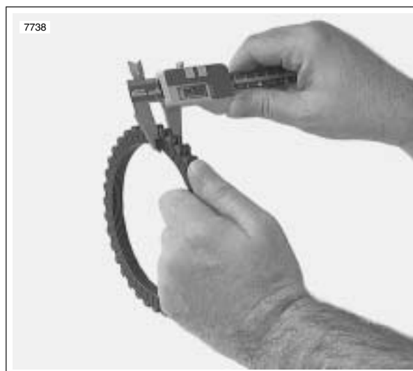
Figure 6-17. Measuring Friction Plates
