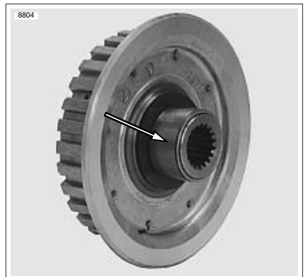
Figure 6-28. Clutch Hub Bearing Race
