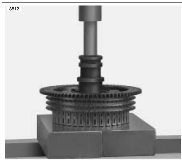
Figure 6-30. Removing Clutch Shell Needle Bearing
