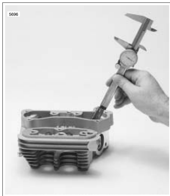
Figure 3-67. Measuring Valve Stem Protrusion
