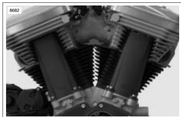
Figure 3-79. Push Rod Locations
