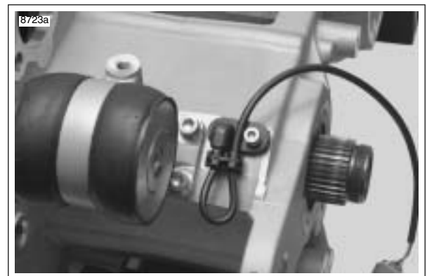
Figure 6-51. Rear Isolator Assembly
