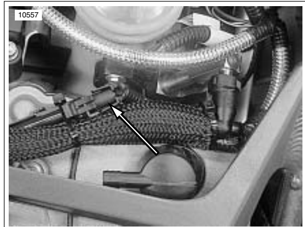
Figure 4-78. Engine Temperature Sensor Connector Approximate Location [90]
