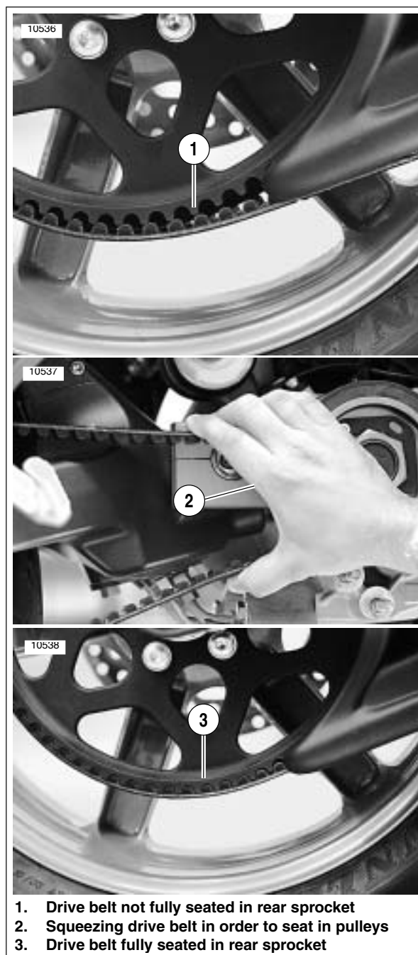
Figure 6-42. Seating Drive Belt Into Pulley Teeth
