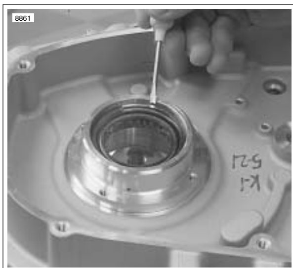
Figure 3-139. Sprocket Shaft Seal Retaining Ring
