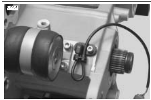
Figure 3-33. Rear Isolator and Mounting Hardware
