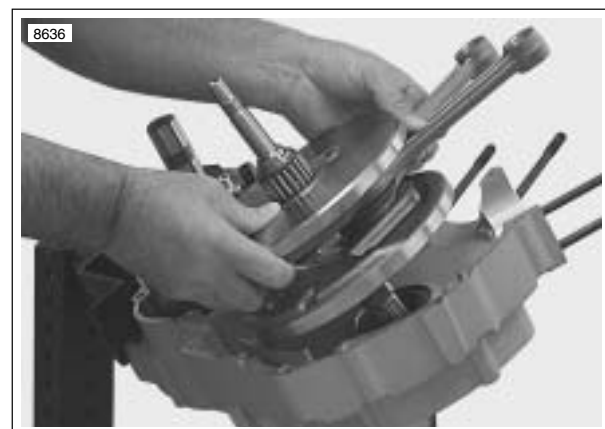
Figure 6-54. Removing Flywheels from Left Case Half
