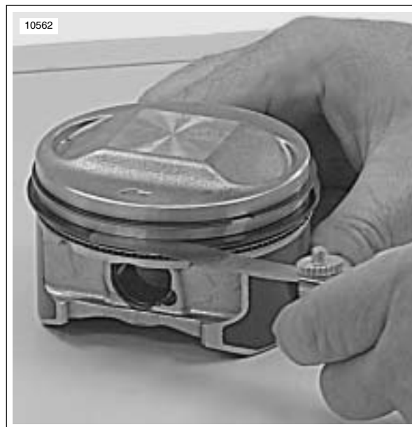
Figure 3-95. Measuring Ring Clearance in Groove
