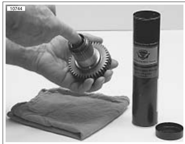
Figure 6-76. Lubricating Main Drive Gear Needle Bearings
