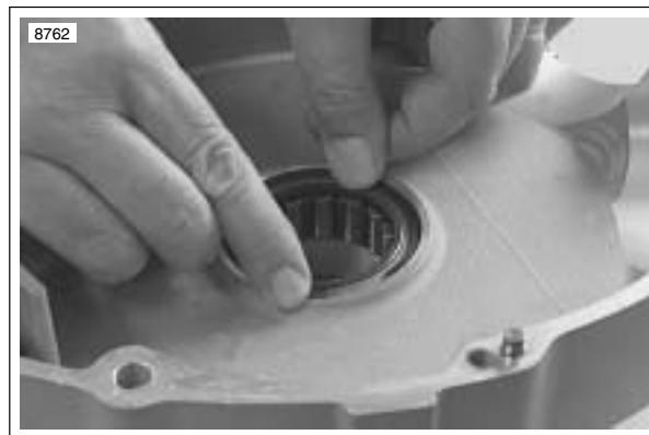
Figure 3-140. Removing Sprocket Shaft Bearing Retaining Ring
