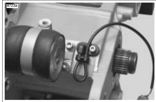
Figure 3-133. Rear Isolator Assembly
