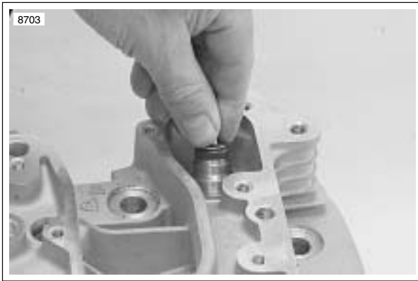
Figure 3-77. Valve Seal and Lower Collar Assembly Installation
