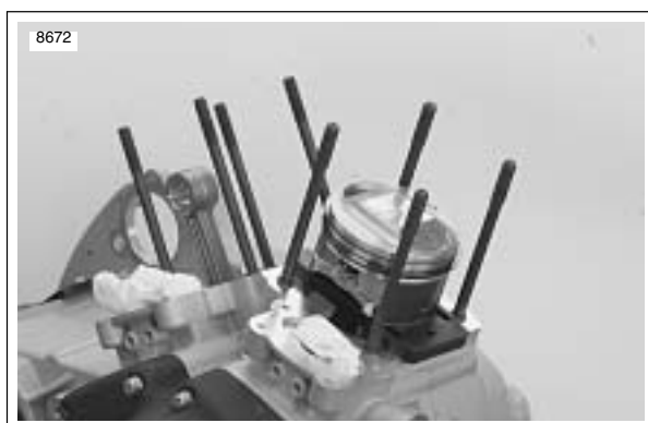
Figure 3-104. Piston Support Plate
