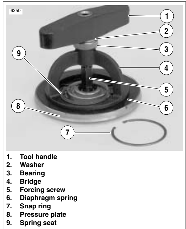
Figure 6-14. Pressure Plate Assembly
