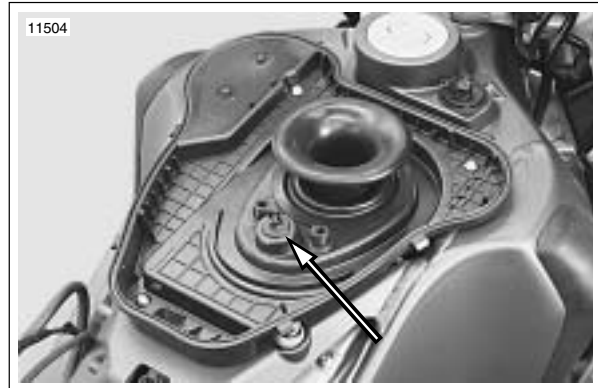
Figure 4-80. Intake Air Temperature Sensor Installed
