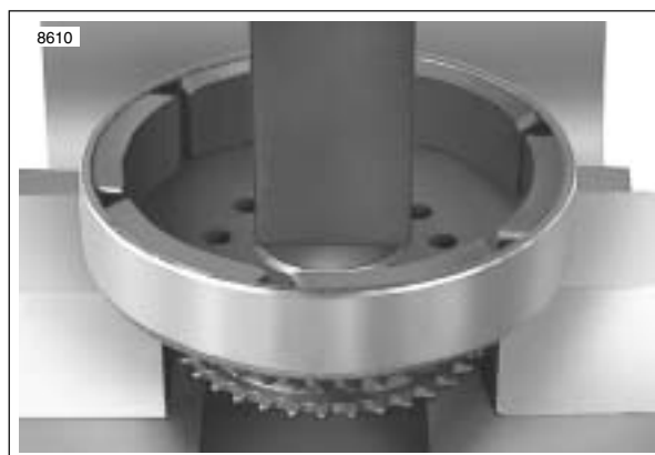
Figure 7-33. Removing Rotor From Sprocket
