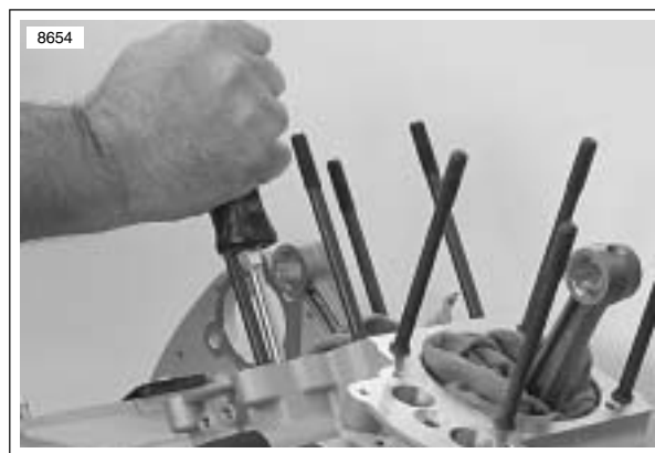
Figure 3-132. Checking Cam Gear End Play
