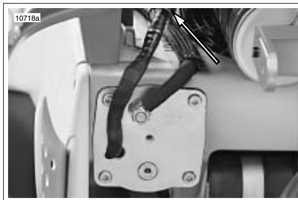
Figure 4-99. Fuel Pump Connector [86] (swingarm removed for illustration)
