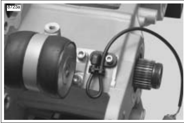
Figure 3-30. Rear Isolator and Mounting Hardware
